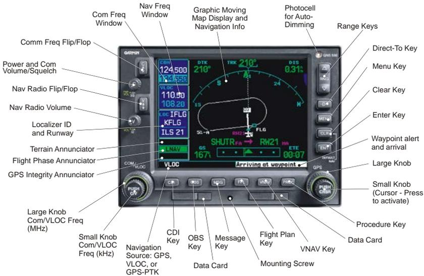
**Figure 1 - 530W Series Control and Display Layout**
