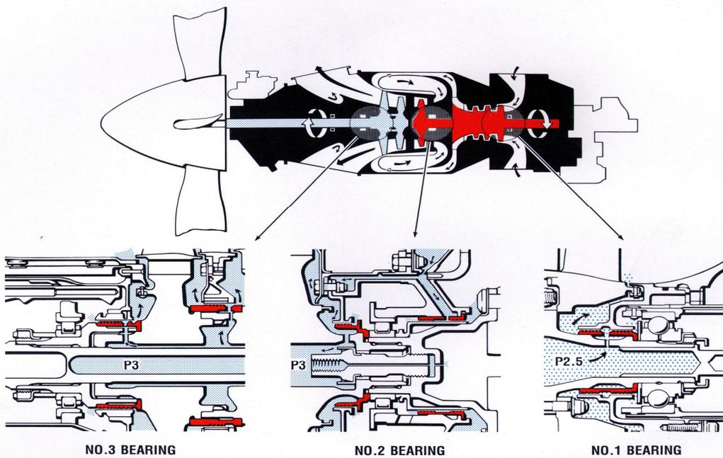
**BEARING COMPARTMENT SEALING**
