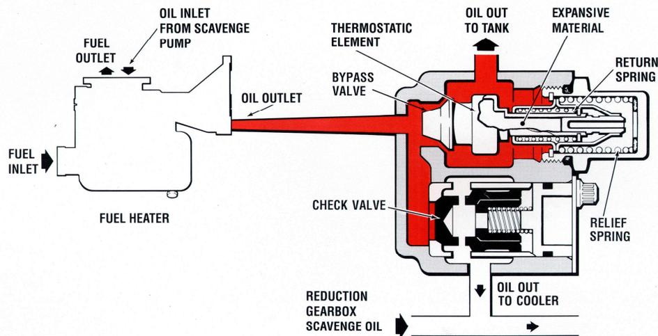
**THERMOSTATIC BYPASS AND CHECK VALVE**
