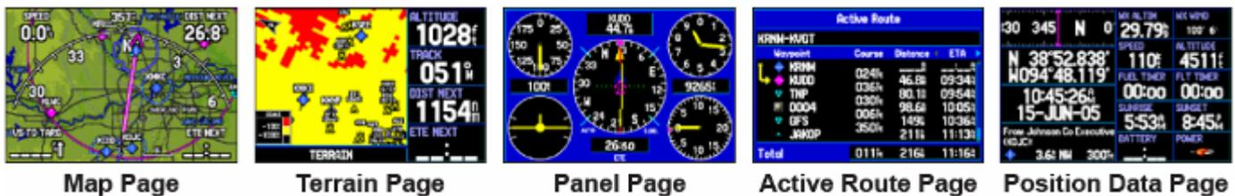
A particular safety feature –and very relevant for eVFR- is the terrain map with the obstacle warning. The obstacle warning automatically pops up in the left bottom corner of other pages as shown below in the panel page (which emulates the traditional instrument panel, serving as a backup).
