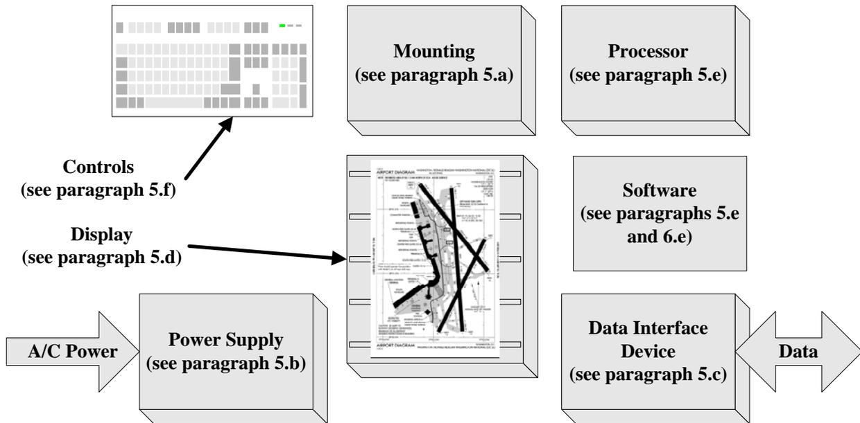
**c. Airworthiness Applicability.** Airworthiness regulations apply to installed EFB components. They do not apply to portable EFB components other than for specifications associated with the installed components (i.e., mounting (size and weight), power (maximum electrical load), and data connectivity (input/output specifications and security)).
