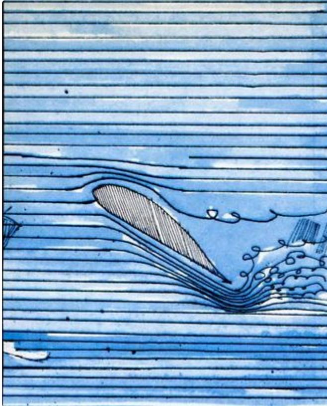
From that stagnation-point position, the air no longer can turn the corner around the leading edge and still have sufficient energy to negotiate the route along the airfoil's upper surface. Being unable to follow the shape of the airfoil, the air separates from its normal path and cannot produce the velocity distribution over the upper surface that is needed to generate lift.
