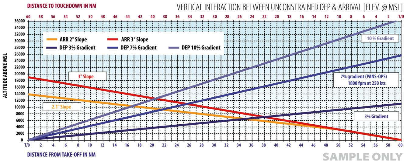
For example: if a departure on a 7% climb gradient (marked on graph) had travelled 25 track miles from the departure end of the runway (read on lower X axis) when it crossed the arrival on a 3° slope which was at 35 track miles from the runway (read on upper X axis), both aircraft would be in the region of 11,000 feet AMSL. So choosing this crossing point would not be efficient because it would restrict the departure's continuous climb and the arrival's continuous descent.
