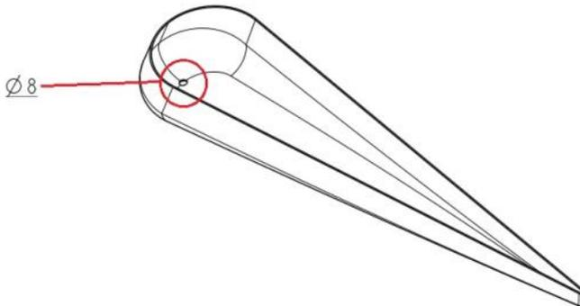
Figure 7-3 Draining system – bottom rudder fairing
