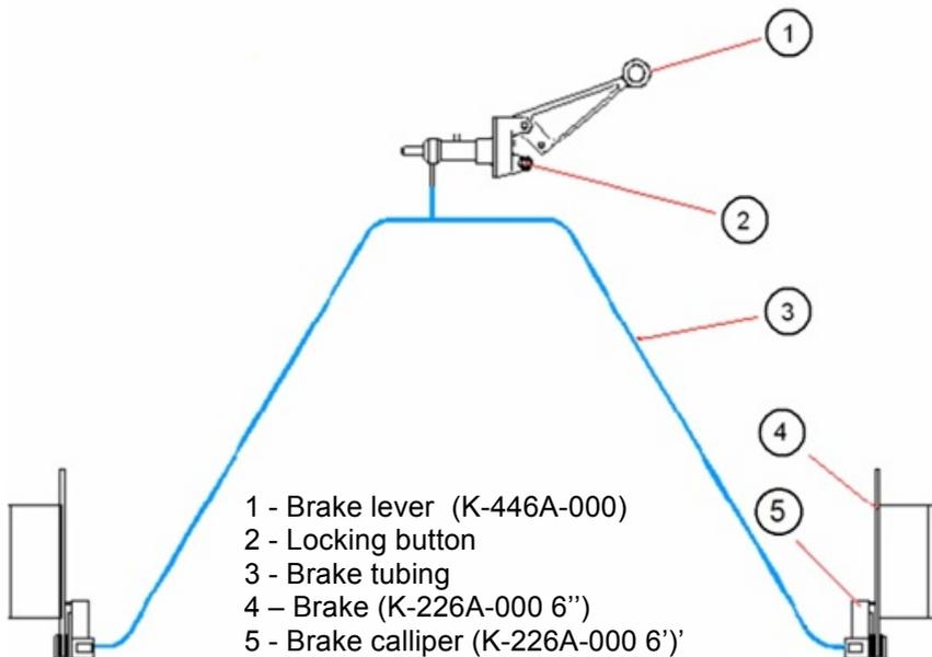
Figure 7-13 Braking system diagram
