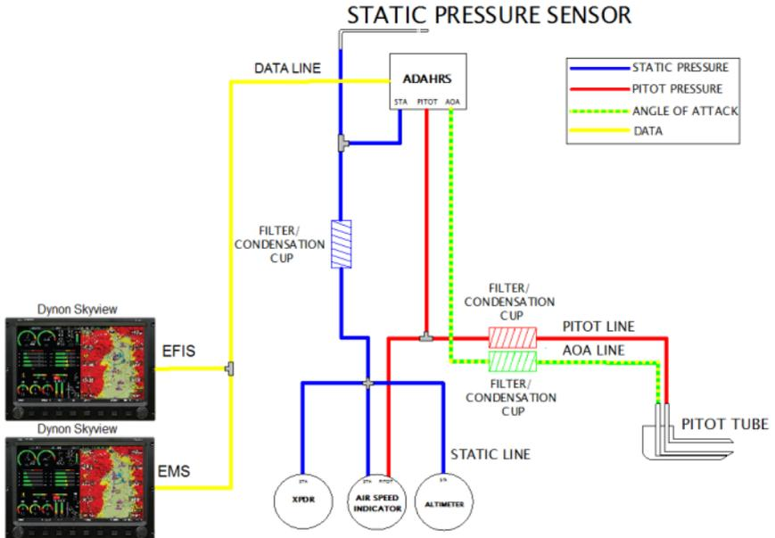
Figure7-14 Pitot-static diagram
