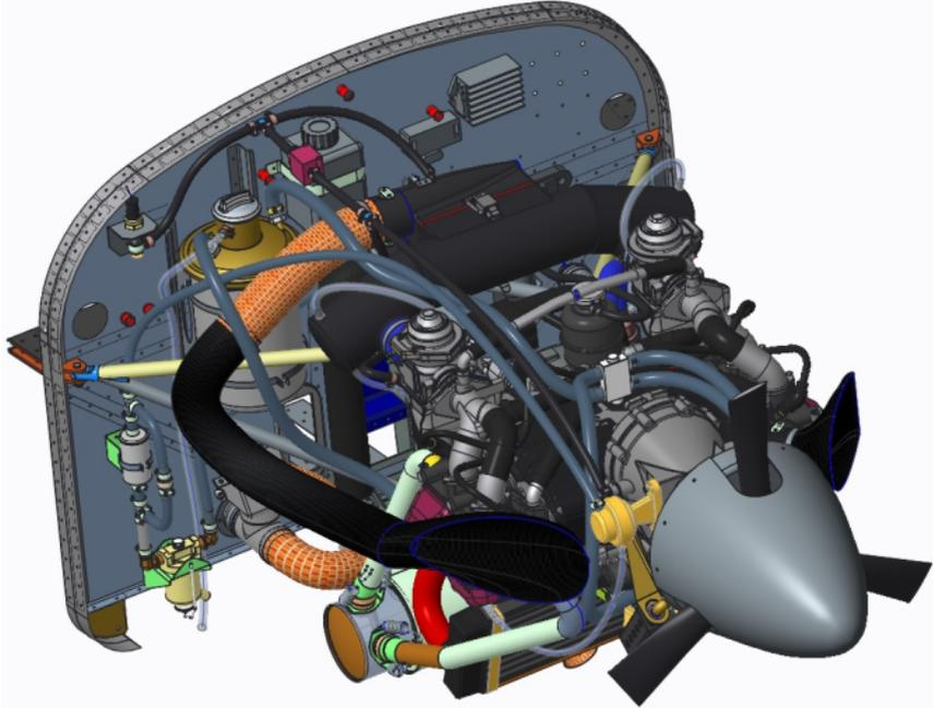
Figure 7-8 Engine unit and airbox air flow
