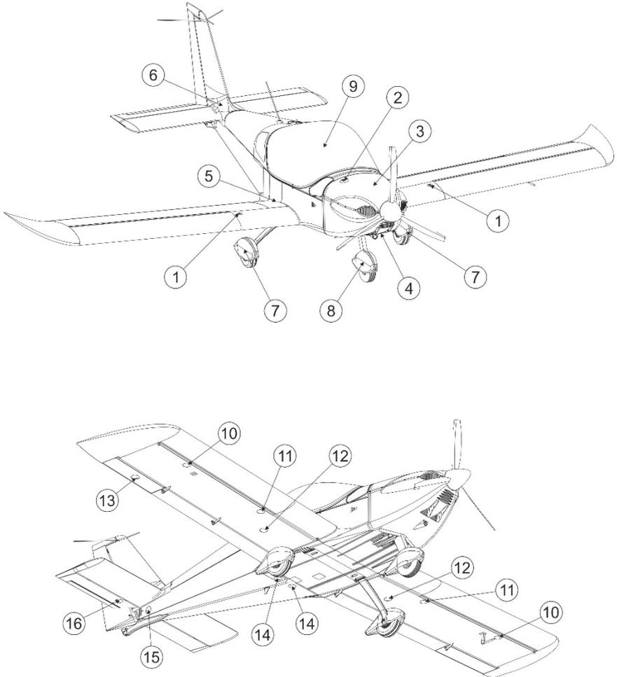
Figure 7-5 Access hatches
