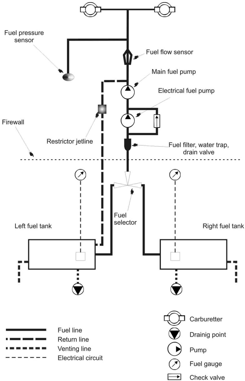
Figure 7-12 Fuel system diagram
