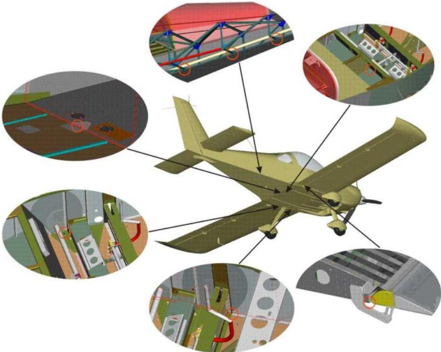
Figure 7-1 Draining system – fuselage
