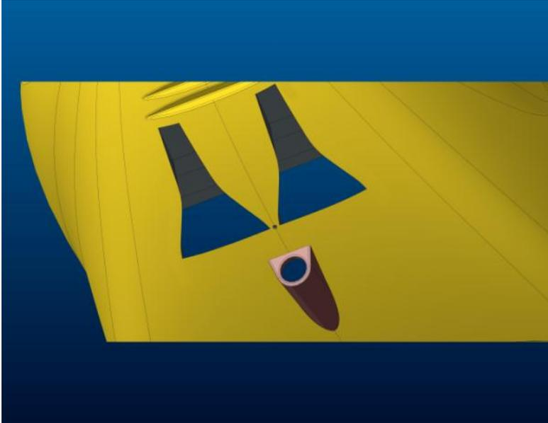
Figure 7-2 Draining system – lower engine cowling – hole between air inlets
