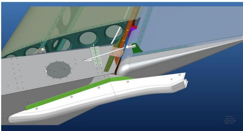
Figure 7-4 Draining system – tail skid aerodynamic fairing
