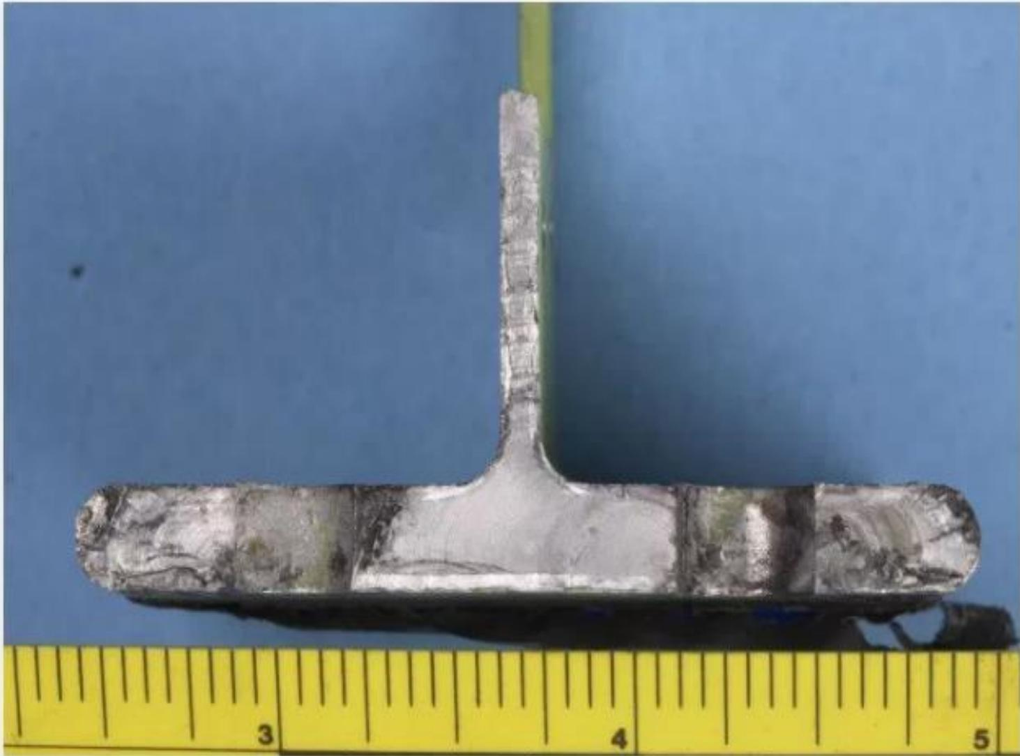
Figure 1 - Left wing main spar lower cap fracture surface.
