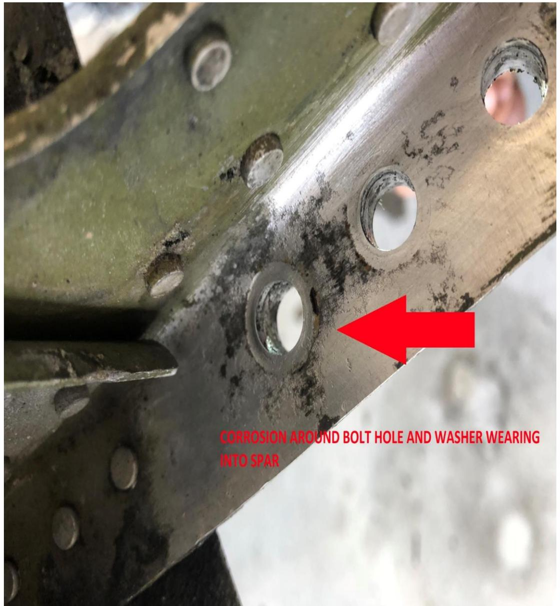
**CORROSION AROUND BOLT HOLE AND WASHER WEARING INTO SPAR**
