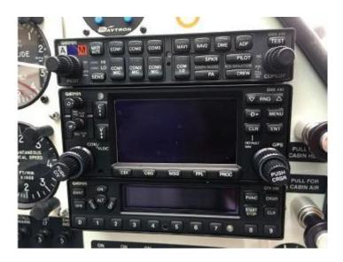
This radio and GPS stack is installed in an Aviat Husky - the sort of kit to be found in up-to-date SEPs with panel GPS.
