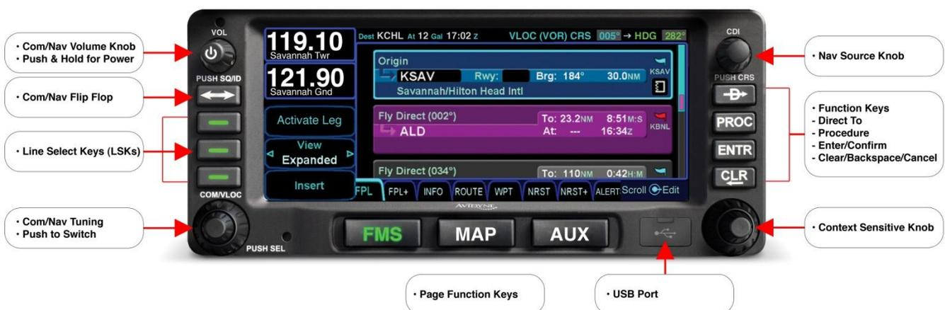
\*The IFD410 does not contain a VHF nav/com radio and therefore does not have a volume knob, flip/flop button, Com/Nav push knob.
