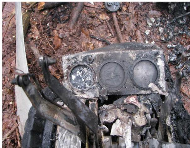
Middle console with engine levers and instruments
