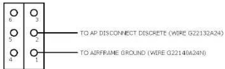
**Figure A-8 – Disconnect Switch Wiring**
