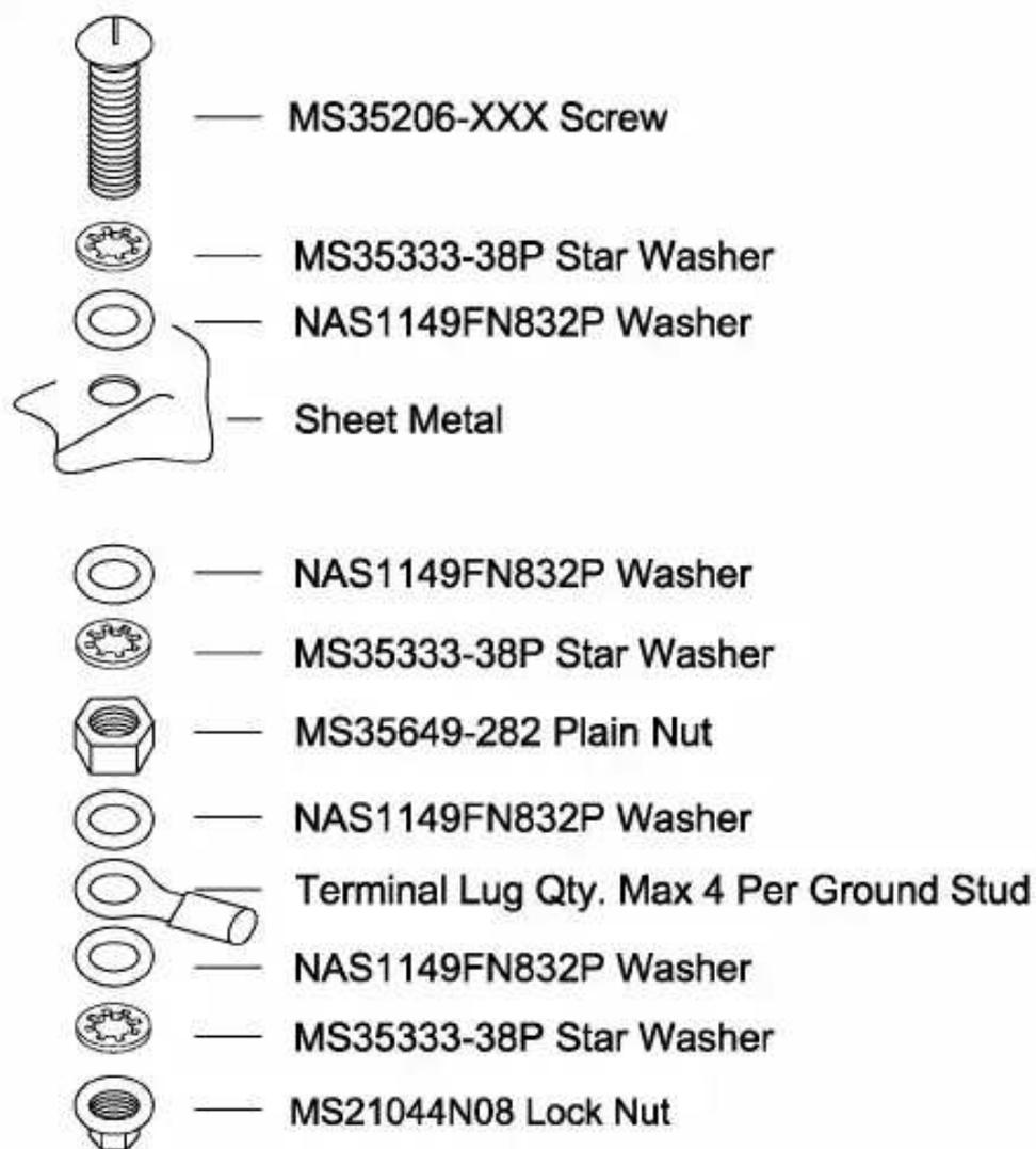
Figure 4-4 – Ground Stud Build Up
