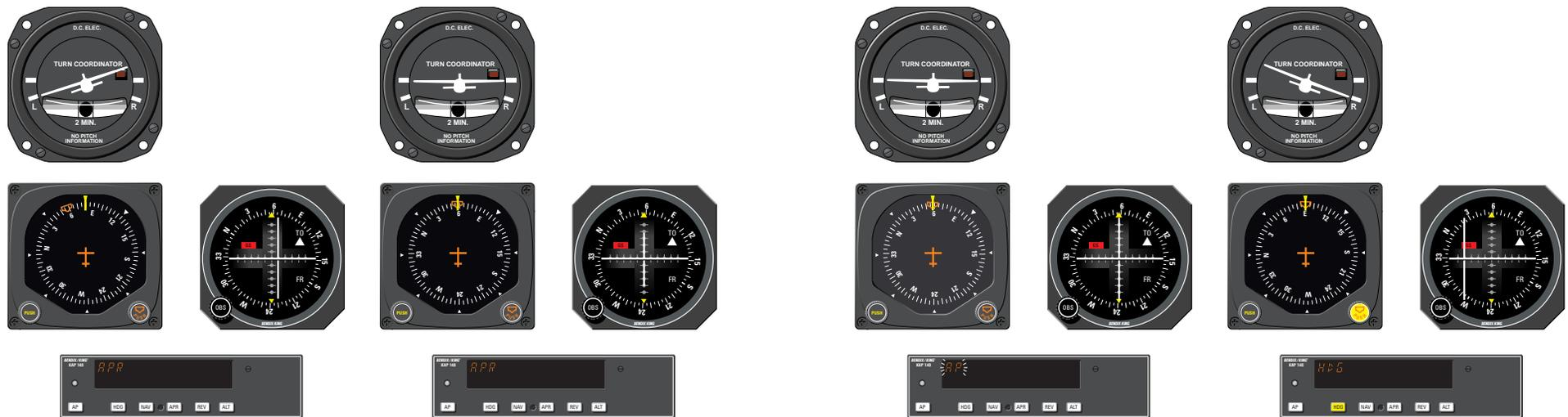
1. Continuing the maneuver on page 46, **APR** mode capture occurs. The autopilot initiates a left turn to track the 058° GPS course. Approach active is indicated on the GPS annunciator.\*
