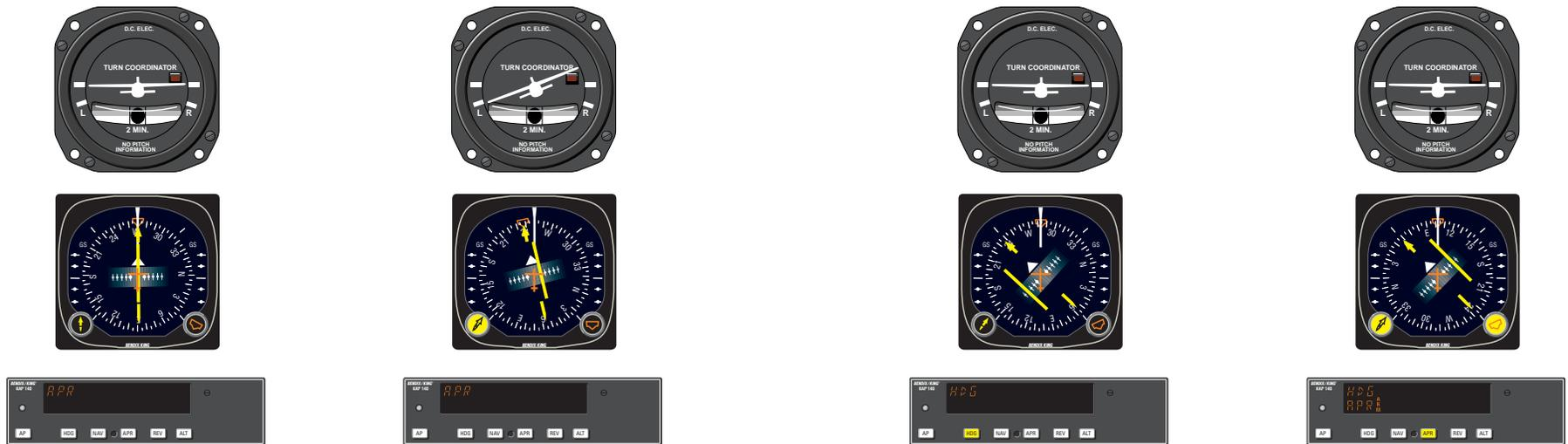
1. The aircraft is in **APR** mode approaching the IAF. Approach arm is indicated on the GPS annunciator.\*
