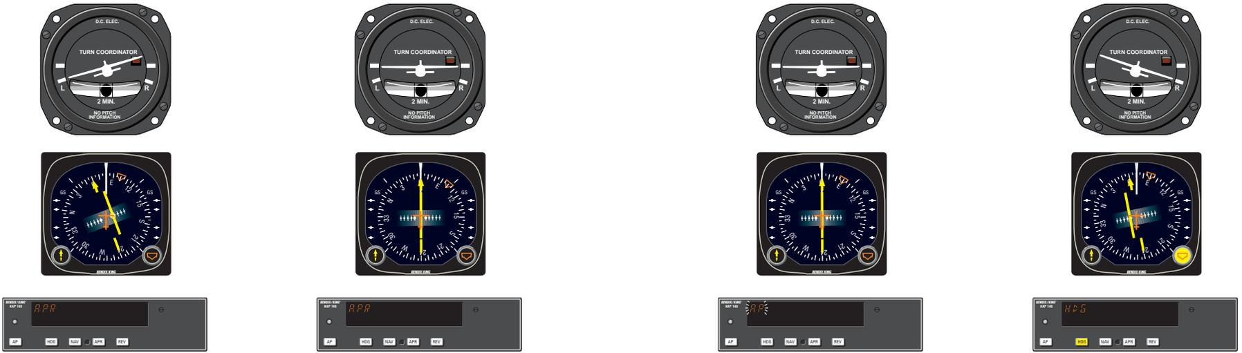
1. Continuing the maneuver on page 40, APR coupling occurs (**HDG** annunciation changes to **APR**). The autopilot will capture the localizer and the CDI course index will center.
