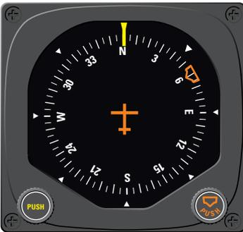
3. If you move the heading “bug” again while the heading select mode is engaged, the autopilot will immediately turn the aircraft in the direction of the newly selected heading.
