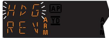
*NOTE: When REV is selected, the autopilot will flash HDG for 5 seconds to remind the pilot to reset the HDG bug to the front course inbound heading. Check the heading displayed on the DG against the magnetic compass and reset if necessary.*
