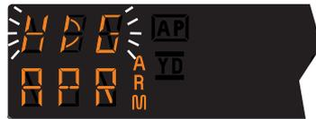
*NOTE: When **APR** is selected, the autopilot will flash **HDG** for 5 seconds to remind the pilot to reset the HDG bug to the desired approach course. Check the heading displayed on the DG against the magnetic compass and reset if necessary.*
