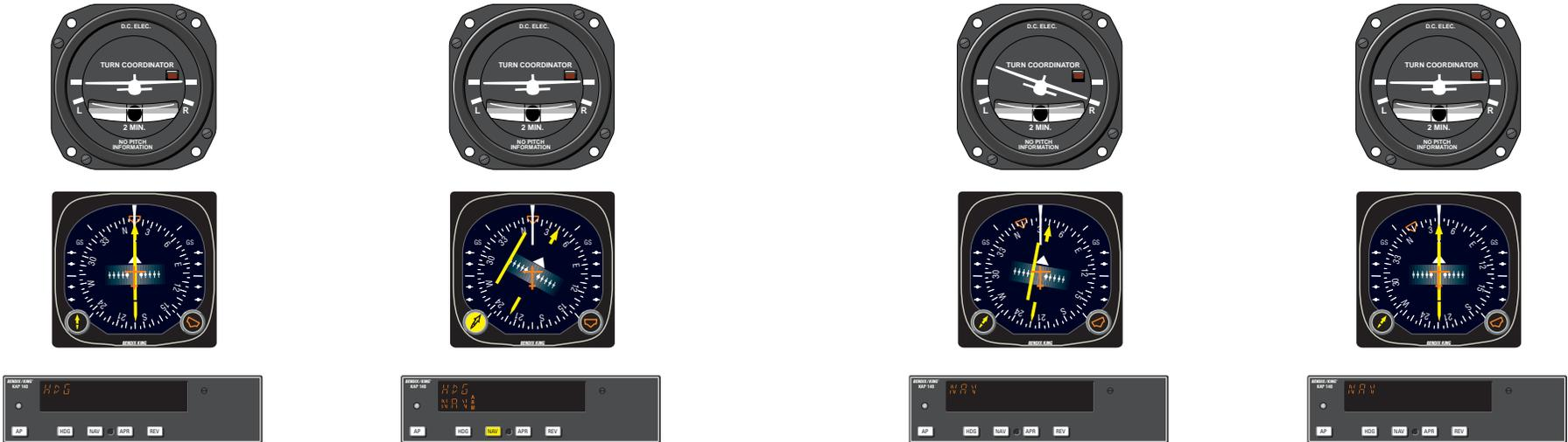
1. Continuing on heading 010°, a GPS waypoint is established. A 30° intercept is desired.
