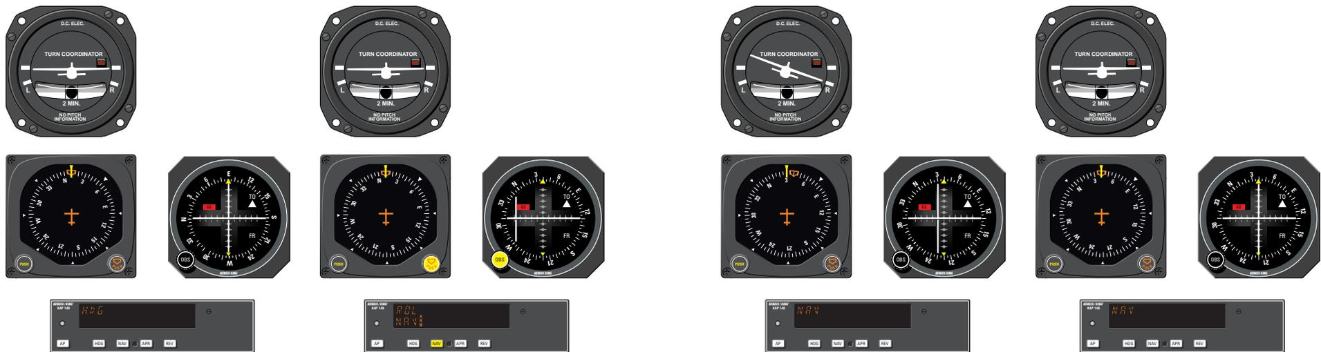
1. Continuing on heading 010°, a GPS waypoint is established. A 30° intercept is desired.
