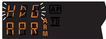
*NOTE: When APR is selected, the autopilot will flash HDG for 5 seconds to remind the pilot to reset the HDG bug to the desired approach course. Check the heading displayed on the DG against the magnetic compass and reset if necessary.*
