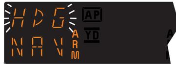
*NOTE: When NAV is selected, the autopilot will flash HDG for 5 seconds to remind the pilot to reset the HDG bug to the OBS course. Check the heading displayed on the DG against the magnetic compass and reset if necessary.*
