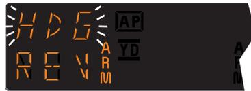
*NOTE: When REV is selected, the autopilot will flash HDG for 5 seconds to remind the pilot to reset the HDG bug to the front course inbound heading. Check the heading displayed on the DG against the magnetic compass and reset if necessary.*
